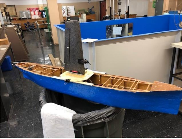
Figure 1. Propeller-Sail remote-control model
