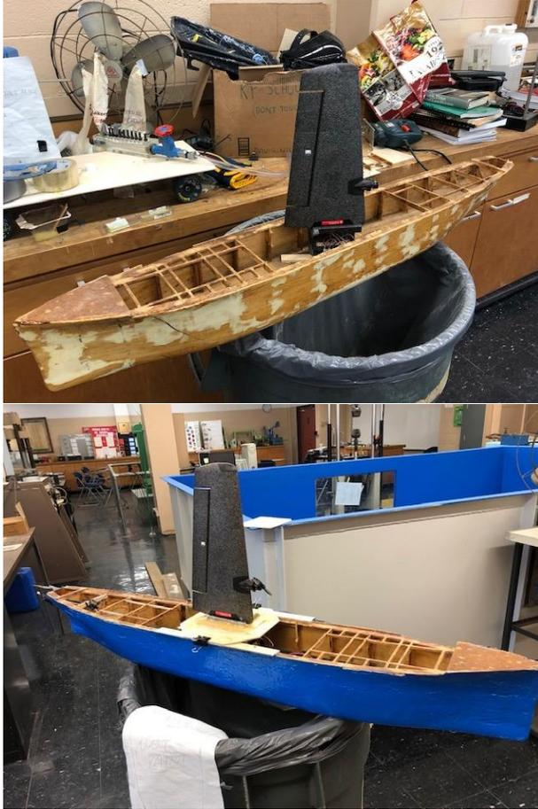
Figure 15. Ship Model before- and after full assembly. Lower figure shows remote controlled rudder and propeller. The aileron was not used in tests.
